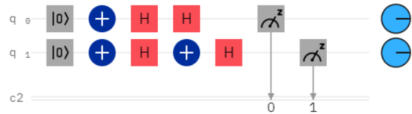
Fig. 12 The implemented circuit for the Constant-1 test
