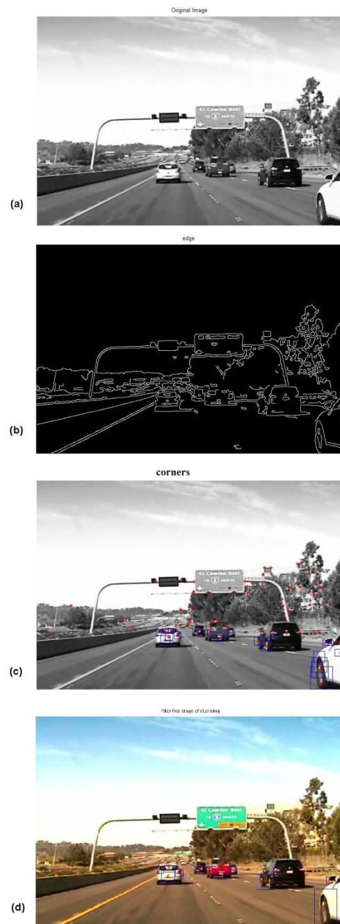
Fig.1. Original image and extracted features (a) original image (b) image edge extracted by canny algorithm (c) corners extracted by harris method (d) adaptive boundingbox
