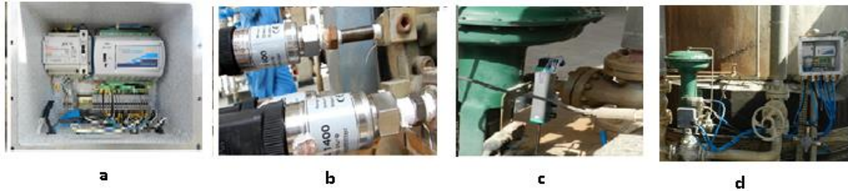
Fig. 2 a: Data logger b: Pressure/Flow transducer c: Rod displacement d: real control valve with all associated sensors
