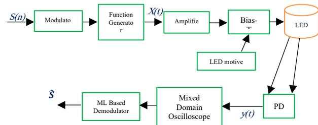
Fig 1: Demodulation based on ML of VLC [9].
