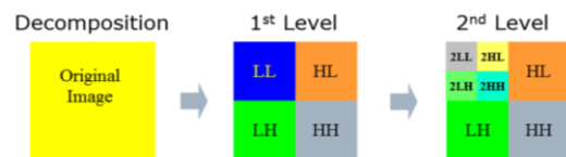
Figure 2: Bands of wavelet transform to the level 2
