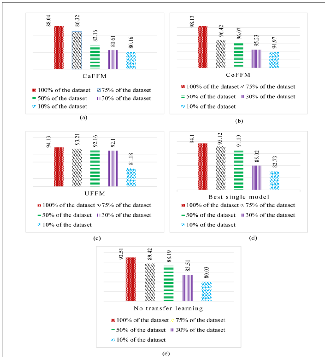
Fig. 4. Accuracy rates of the proposed methods on the IDSAI dataset for detecting unknown attacks
