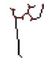
Fig. 5 Skeleton of a sample digit '3' with its branch points represented by red spots; #BP = 7 [43].
